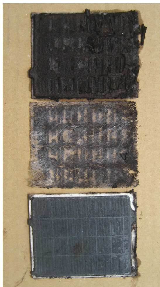
Fig. 2: Electrodes from top to bottom: Lead dioxide comb, Diaphragm, Metallic lead plate.
