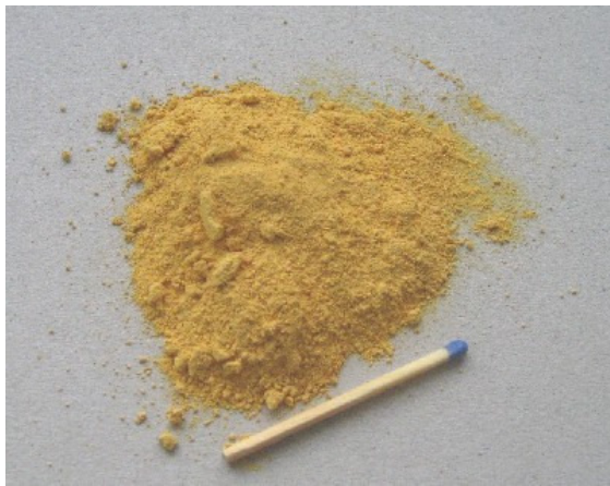
Fig. 3: Yellow lead oxide, 35 grams, enough for making 700 ml of 5% lead acetate solution for impregnating many meters of match cord.
