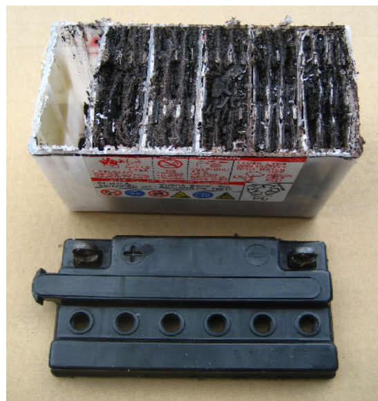
Fig. 1: The decapitated battery, exposing electrodes.
